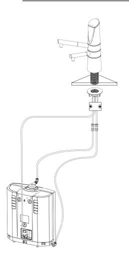
The ECAIA ionizer S+ can be permanently connected to the angle valve under the sink, as described under point "1.4 - Permanent connection to the angle valve (appliance in above-counter position)". Due to the positioning of the device under the sink, it must be operated using the special ECAIA ionizer S faucet. A solenoid valve must also be interconnected to control the water supply.
