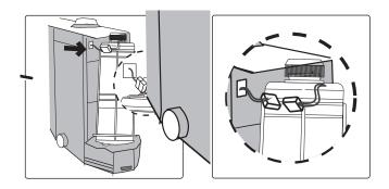
3. Turn the filter counterclockwise and remove it by pulling the filter up and out. The residual water may flow out of the filter or the device. Dry excess water with a clean, absorbent cloth. Excess water can penetrate inside the device.
