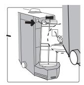
7. Place the filter cover (B-4) in the place provided on the device and slide it down until it clicks into place. If the filter cover does not click into place, release the fixing on the filter cover lock button.
