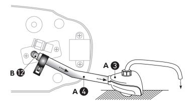
**Note:** Make sure that the alkaline outlet hose (A-2) or the stainless steel spout from the acidic water tap (A-3) do not come into contact with dirty objects. Likewise, the plastic hose for acidic water 7/9 mm (A-4) should not be connected directly to the drain. This could cause re-contamination of the device.
