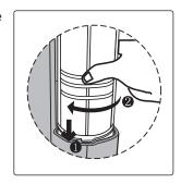
6. Connect the plug lock on the filter cable.
