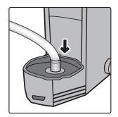
5. Connect the descaling pump to the power supply. The pump starts automatically.
