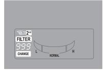
**Note**: If the filter is not changed, even though the maximum flow rate has been reached, the device will not switch on immediately. The display will not switch on until a new filter has been inserted, regardless of the water flow.
