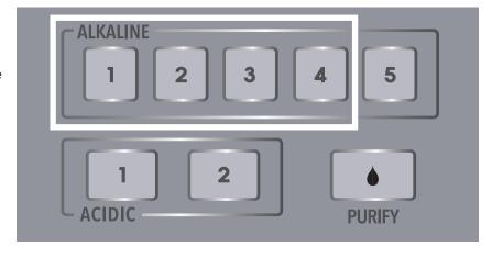
**Example**: You select the alkaline level 3 and then switch off the device. The next time you switch on the device, alkaline level 3 is automatically selected again.
