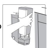
2. Disconnect the plug lock on the filter cable.
