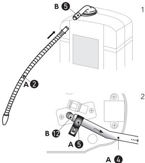
1. Screw the alkaline outlet hose (A-2) to the upper water outlet (B-5).
