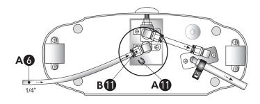
5. The water pressure can be adjusted with the adjustment screw on the T-piece (A-10).
